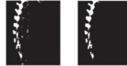
Fig.7. Output Binary image from density based (Left image) and Output from area opening Morphological transformation (Right image)
