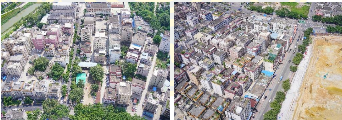
Figure 11. Example of two nearest images in the same flying direction, with underline an approximated overlapping area.
