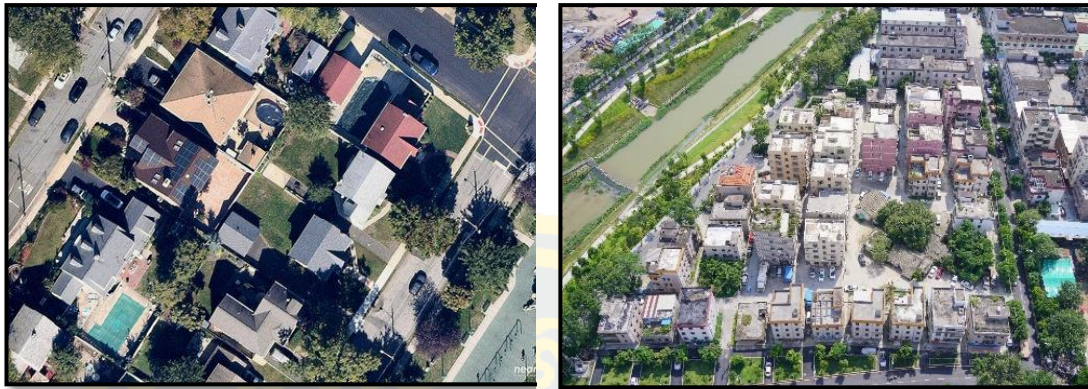
Figure 4. General of Aerial Image, the nadir axis can snap only the top of the building (left). The oblique imagery provided to snap the side of the building (right). ( https://geozoneblog.wordpress.com/2016/03/28/oblique-images-a-tool-you-need/ )
