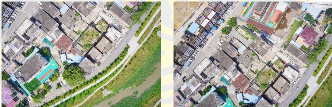
Figure 13. A photogrammetric survey of the urban area displayed overlapping of two images. It used for the Dense Image Matching algorithm process.
